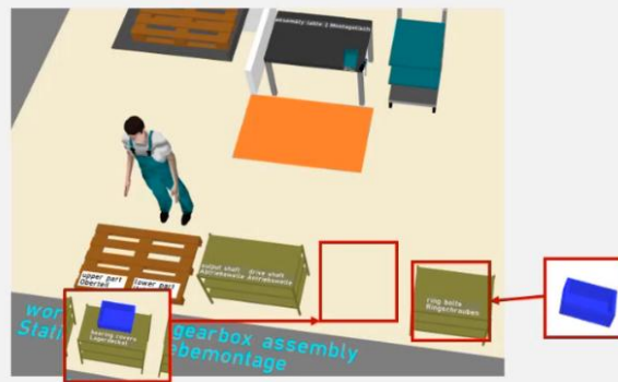
Figure 5.1. Virtual workstation model with a digital human simulation in Ema Work Designer.
