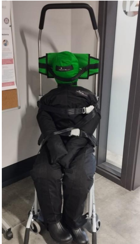
Fig. 3.1. Evacuation chair used for the safe transport of people with reduced mobility during emergency situations.
